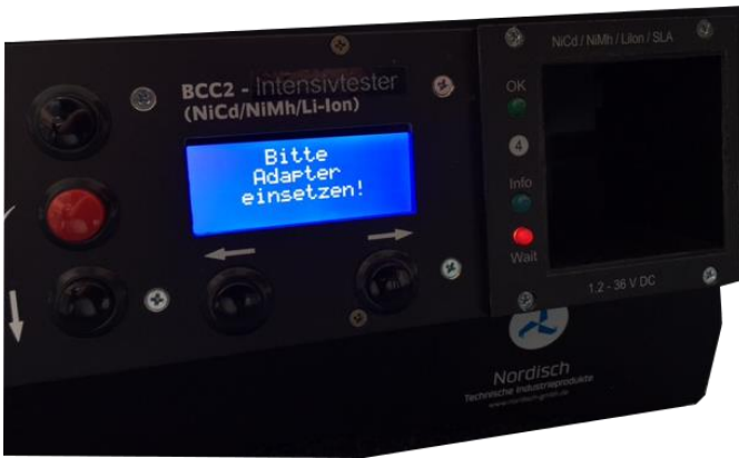
Figure -3, BCC2: Signal encoding without inserted adapter
